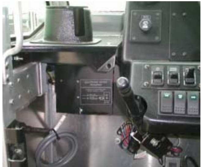
Figure BA-25 Chassis fuses to the left of the dash panel.
