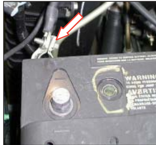
Figure BA-20 Negative (black) Cable Disconnected and Tucked Away
