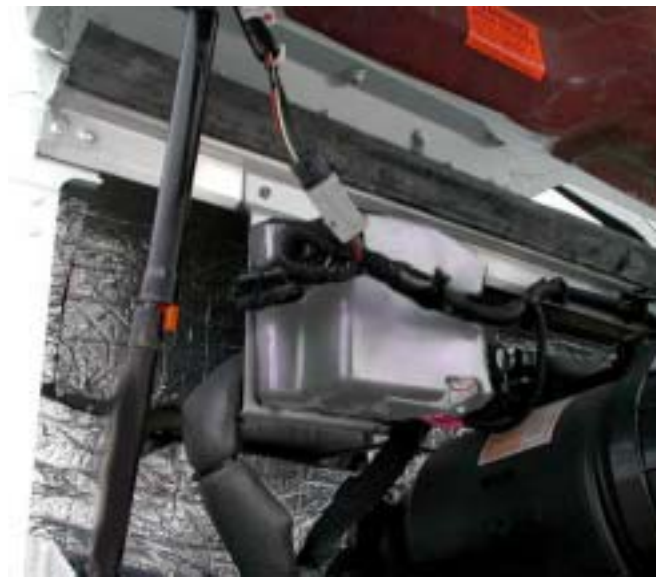
Figure BA-30 Chassis fuses under the hood on the right-hand (passenger's) side of the vehicle.
