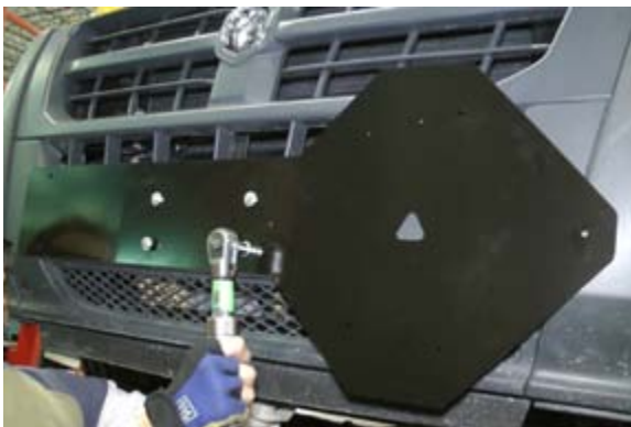
Bumper bracket fasteners
