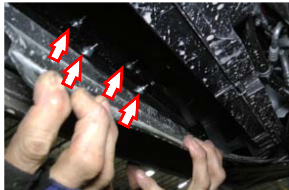
1/4-20 nuts and washers (view from under bumper)
