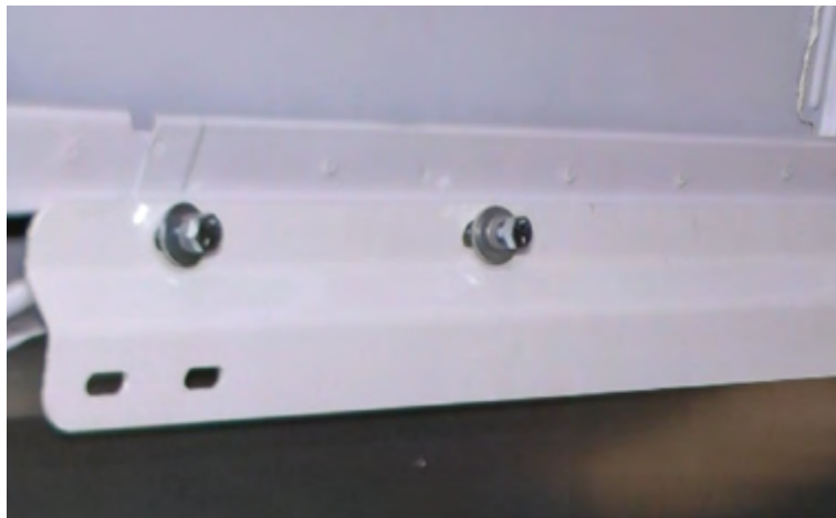
Rail installed with M8 fastener
