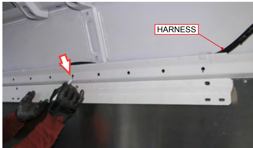
Align sidewall hex holes with rail holes
